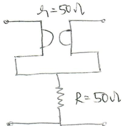
$$Z_{\text{gyrator}} = \begin{bmatrix} 0 & -g \\ g & 0 \end{bmatrix} \quad Z_R = \begin{bmatrix} R & R \\ R & R \end{bmatrix}$$
