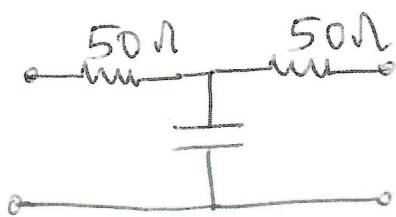
$$Z_a = R + Z = \begin{bmatrix} R + \frac{1}{j\omega C} & j\omega C \\ j\omega C & R + \frac{1}{j\omega C} \end{bmatrix}$$
